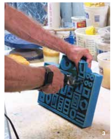
1 The laser cutter in action cutting a 12×12-inch block of sponge. Prior to cutting you will determine the best power and speed of the laser. Always test and determine settings for each machine before cutting. 2 Laser-cut block of Aquazone sponge. This block of sponge will be cut apart into 51 individual stamps. 3 Cut out the individual stamps using an electric serrated kitchen knife.
