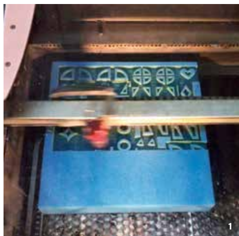
1 The laser cutter in action cutting a 12×12-inch block of sponge. Prior to cutting you will determine the best power and speed of the laser. Always test and determine settings for each machine before cutting. 2 Laser-cut block of Aquazone sponge. This block of sponge will be cut apart into 51 individual stamps. 3 Cut out the individual stamps using an electric serrated kitchen knife.
